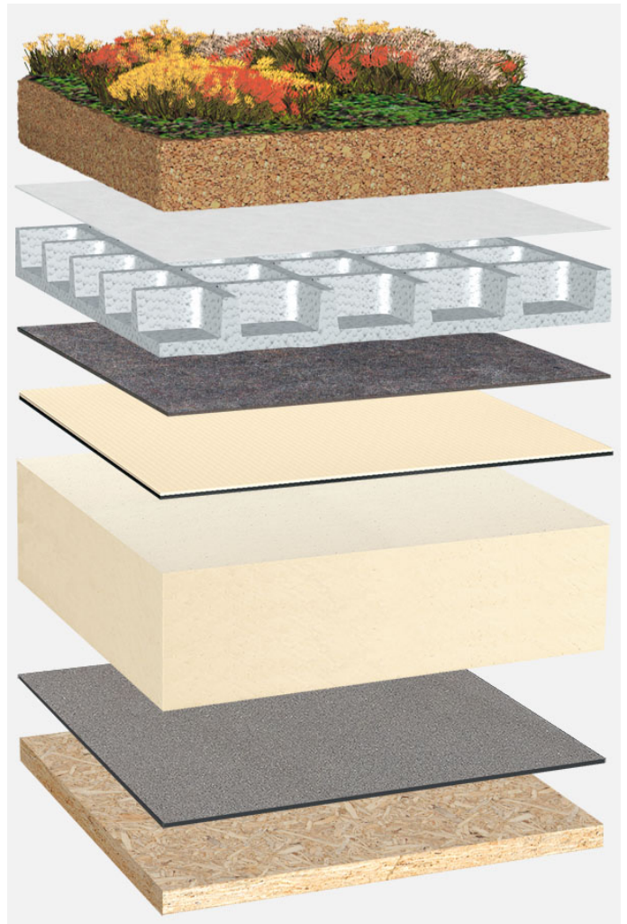
System build-up: HG_PIR-MF_T_01_G75
