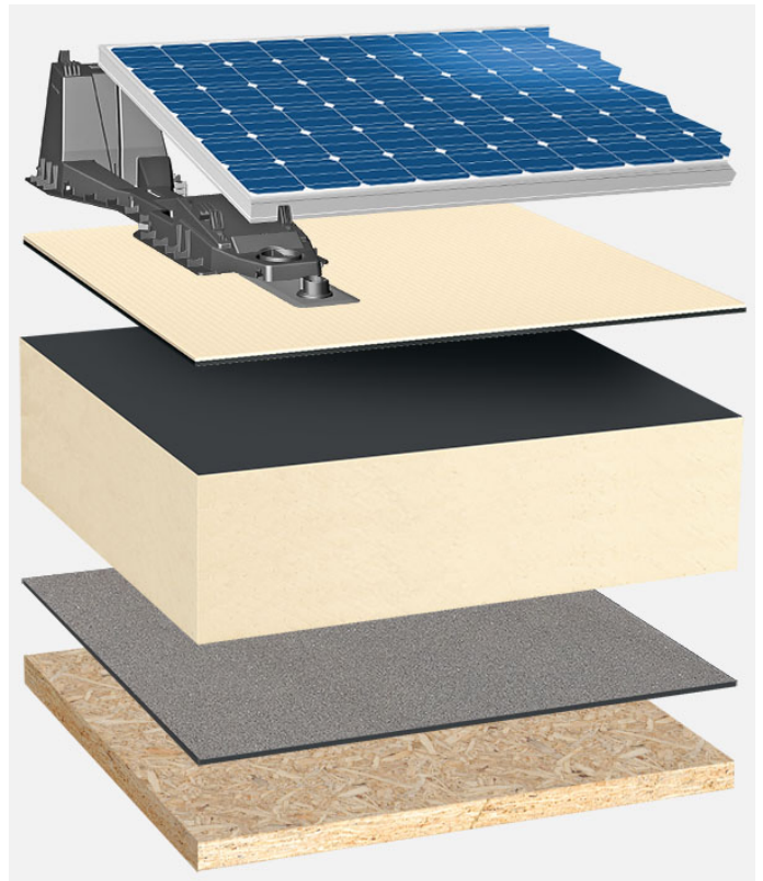
System build-up: HG_PIR-FA_T_01_PVFD
