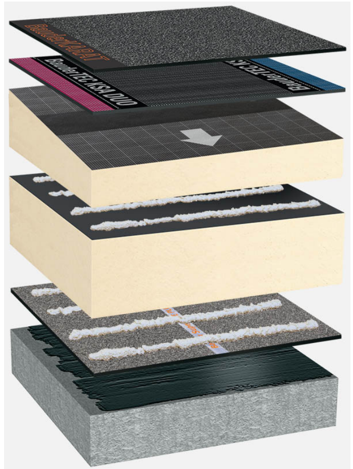
System build-up: BP_PIR-FA_PIR-FAG_K_01
